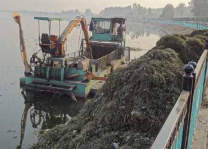
Figure 22. Mechanical removal of Ceratophyllum demersum from Dal Lake of Kashmir by Lake Authority. Photo by : S. Sandilyan
